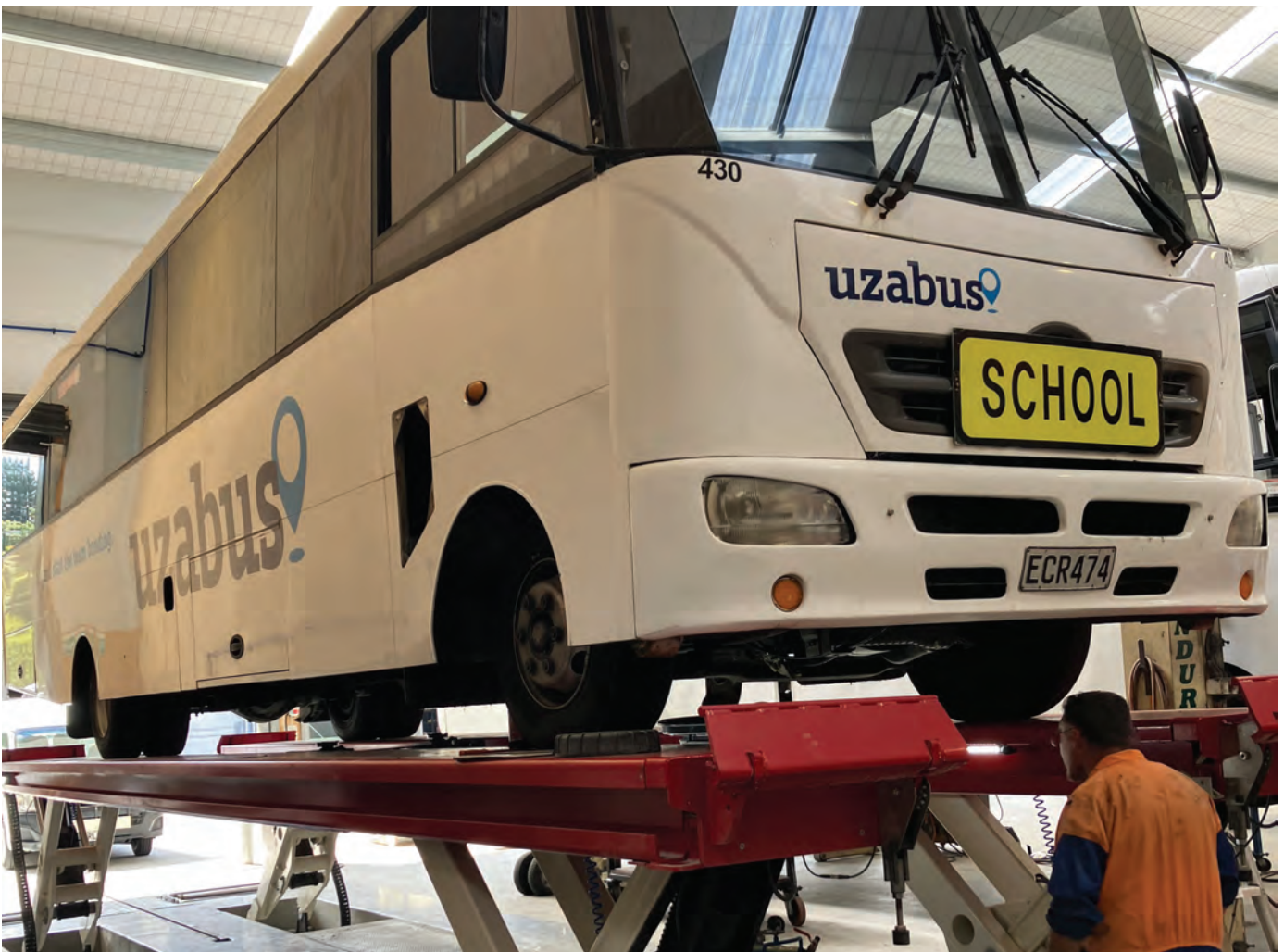
A FLUSH-MOUNTED 'SKY-LIFT' is a feature of the new Uzabus workshop at Tauranga's Tauriko Industrial Estate.
